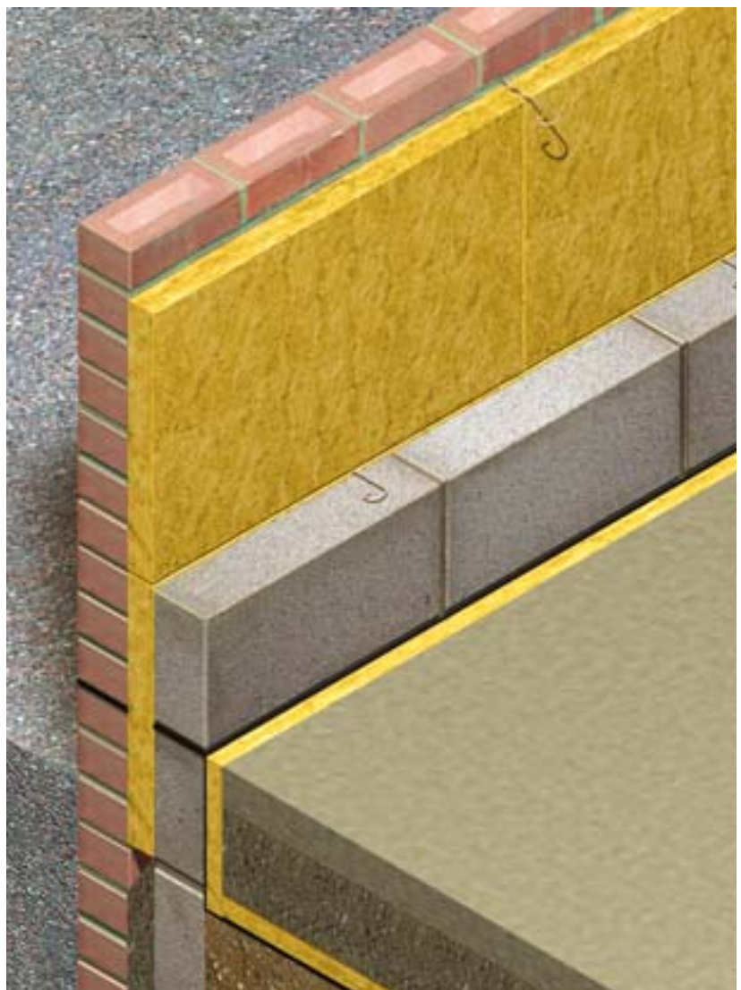
Brick/block wall with second course of batts in place, showing outer leaf raised first and location of wall ties
